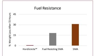
The Hardicrete system shows no degradation when subjected to a chemical attack from diesel or aviation fuel. It has a significantly higher tolerance to fuel than conventional SMA materials.
