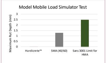
An MMLS Test is designed to imitate real world conditions of accelerated loadings. It measures the impact of moisture, resistance to deformation, longitudinal profile and visual surface condition.
