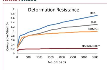
A Cyclic Compression Test under dynamic loading shows Hardicrete™ to have a far superior resistance to permanent deformation than conventional materials.
