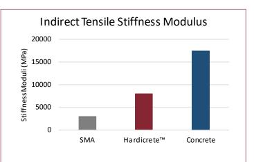
An Indirect Tensile Stiffness test shows deformation and temperature susceptibility. These results were recorded at 20° and show Hardicrete<sup>™</sup> as a hybrid between asphalt and concrete.
