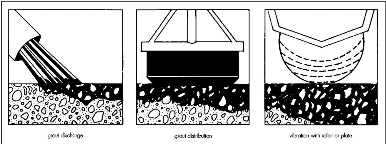
13.5 The receiving course is deemed to be fully penetrated when, following vibration, no further grout can be forced into the voids and surplus grout remains on the surface.
